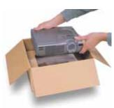
1 At the packaging station, the frame is assembled and placed in the box to suspend the product in the center of the container.
