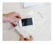
1 The side flaps fold upward, loosening the film and forming an "insertion pocket" for easy product loading.
