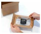
2 When the product is placed in, the flaps are folded down, which tightens the film securely around your product.
