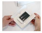
2 The side flaps are folded down to tighten the retention film and hold the product securely in place.
